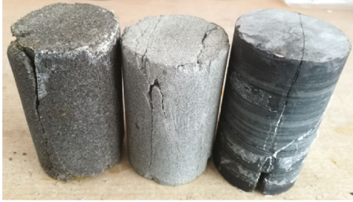
FIGURE 1: Fractured rock specimens (from left to right: coarse-grained sandrock, fine-grained sandrock, and sandy mudrock).
