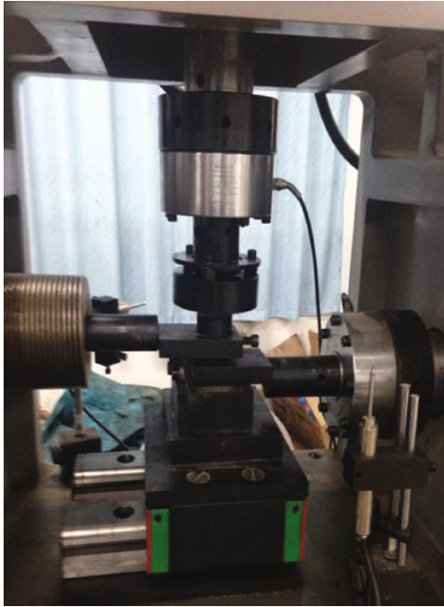
FIGURE 4: The direct shear testing system.
