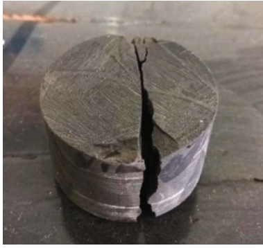
FIGURE 5: The failed specimen in the Brazilian split tests.
