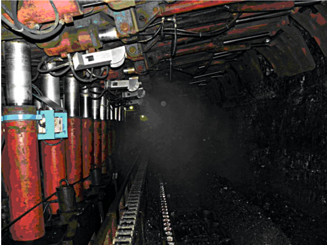
FIGURE 11: Field application diagram of dust collecting device in support shifting operation.
