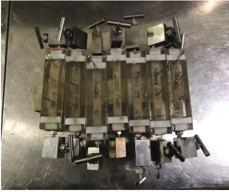
FIGURE 10: Microelectrode core model of different permeability.
