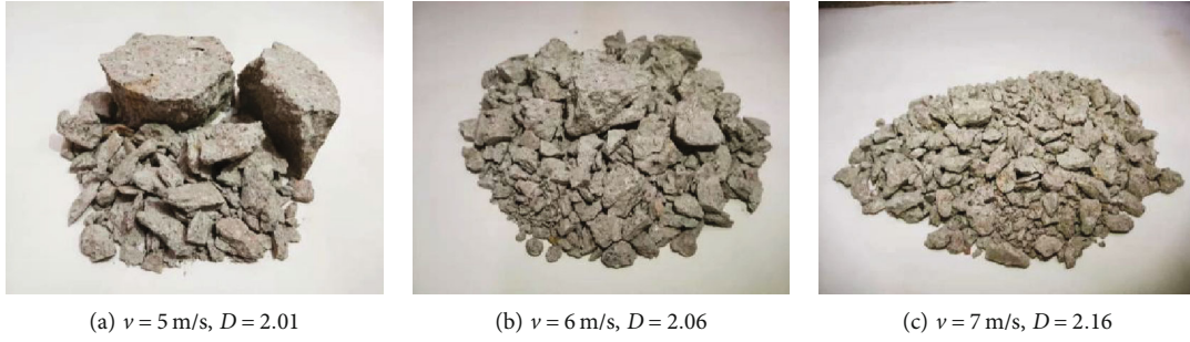
FIGURE 6: Concrete failure morphology at different impact speeds.
