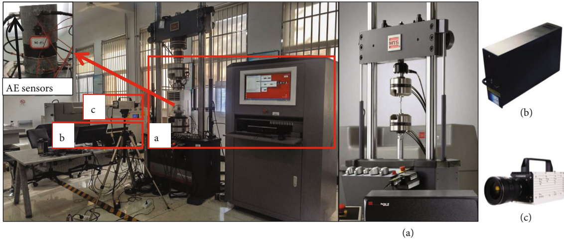
FIGURE 2: Test device and measuring system. (a) MTS Landmark 370.50; (b) PCI-II AE system; (c) NAG GX-3 high-speed camera.
