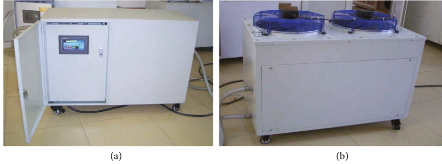
FIGURE 6: Main machine (a) and refrigeration auxiliary machine (b).
