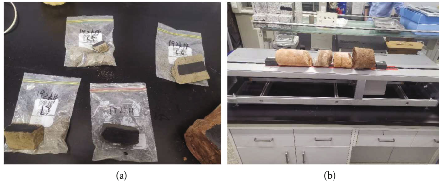
FIGURE 3: Core drilling of K11 and K14 (a) and testing process (b).
