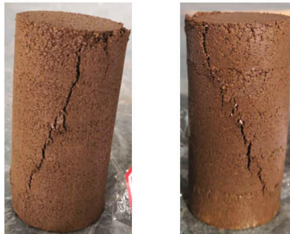
(a) 2% oil content, \rho_d = 1.55 \text{ g/cm}^3 (b) 12% oil content, \rho_d = 1.55 \text{ g/cm}^3
