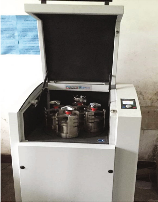
FIGURE 3: Planetary ball mill with four platforms.
