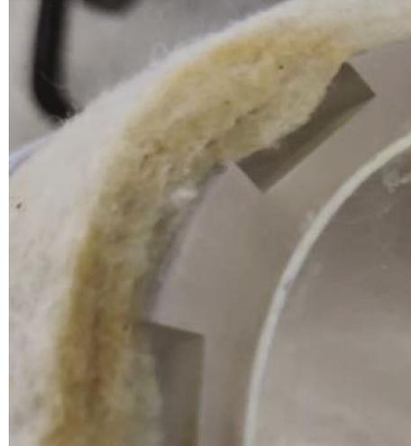
FIGURE 11: Grooves in the direction of the geotextile thickness.
