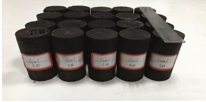
FIGURE 1: Coal samples with different soaking times.
