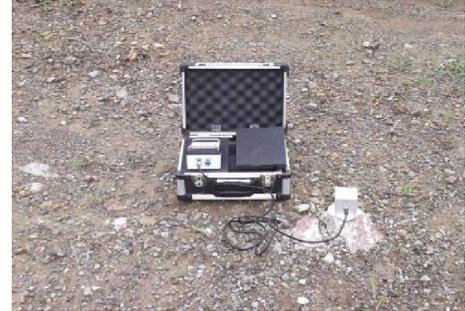
FIGURE 6: TC-4850 blasting vibration tester.
