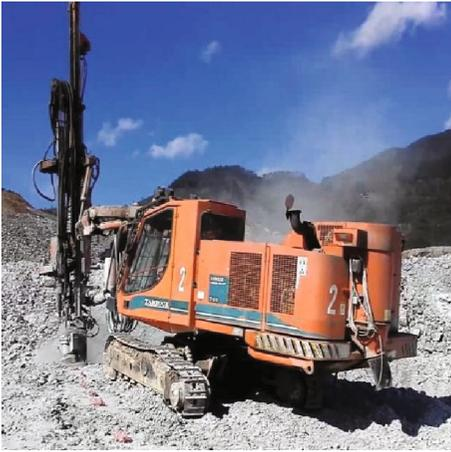
FIGURE 3: Down-the-hole drilling.
