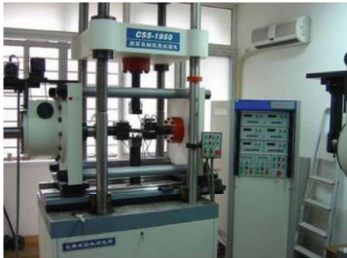
FIGURE 4: CSS-1950 biaxial rheological rock tester.
