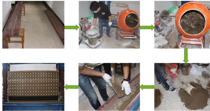
FIGURE 5: Similar material model laying process.
