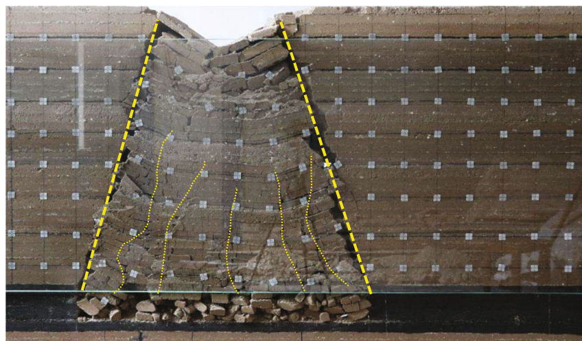
(c) Characteristics of mining fissures after the third layer excavation of section 010202
