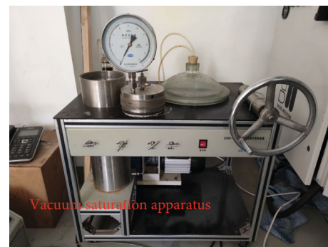
FIGURE 3: The vacuum saturation apparatus for the preflawed samples.
