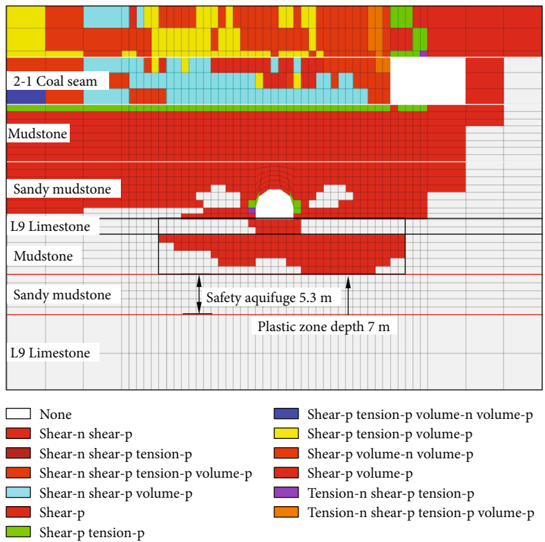
FIGURE 9: Failure of bottom rock stratum at y = 260 m in the floor drainage roadway at an internal stagger of 25 m.
