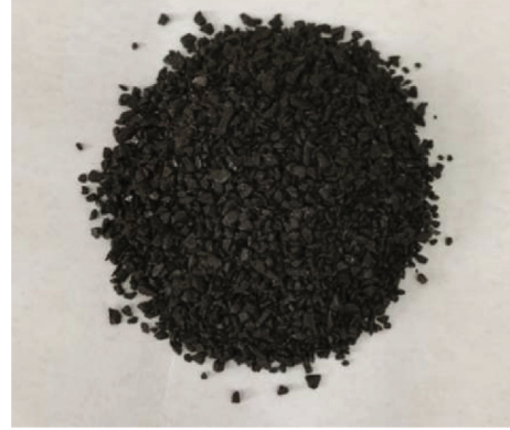
FIGURE 1: Experimental samples (coal particles with the sieving diameter of 1~3 mm).
