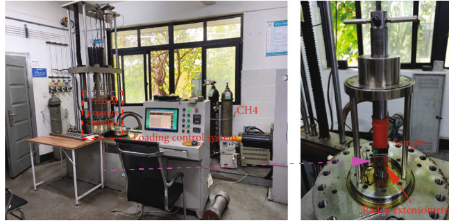
FIGURE 2: Thermal-fluid-solid coupling seepage apparatus for coal and rock containing gas.
