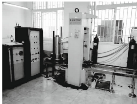
FIGURE 8: RLW-2000M coal and rock rheometer [58].
