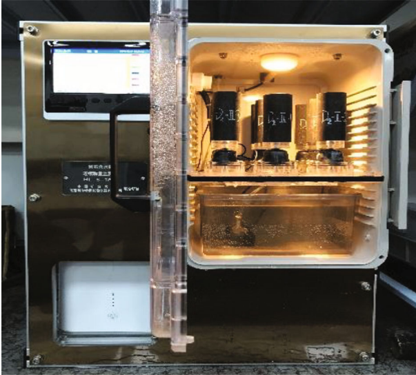
FIGURE 2: Nondestructive immersion device.
