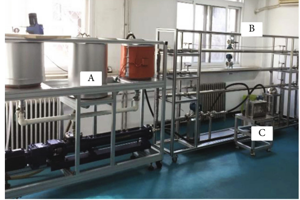
FIGURE 4: Indoor visualization drag testing cycle system: (a) liquid supply system; (b) pipeline test system; (c) visualization fracture model.
