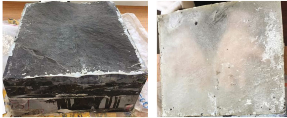
FIGURE 3: Large-scale actual triaxial hydraulic fracturing surface and copied fractures.
