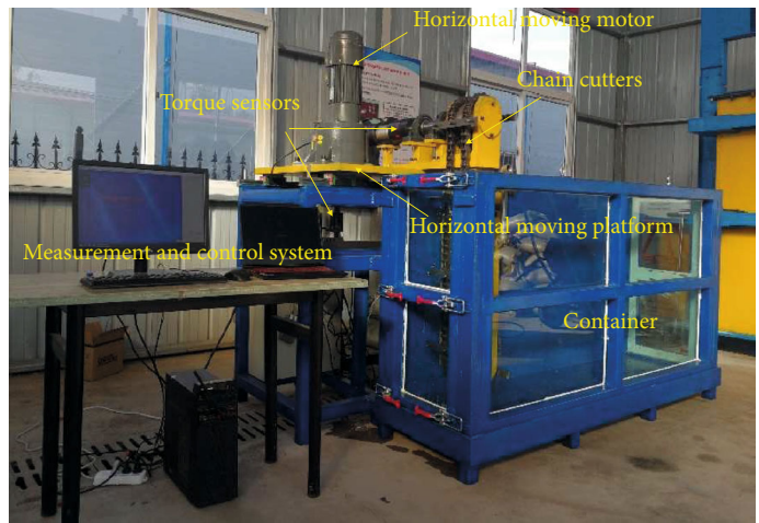
FIGURE 12: TRD model test device [6].
