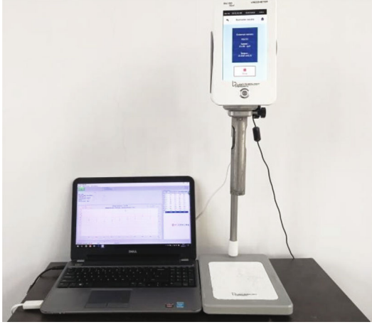
FIGURE 2: Lamy RM100 touch-type rheometer.
