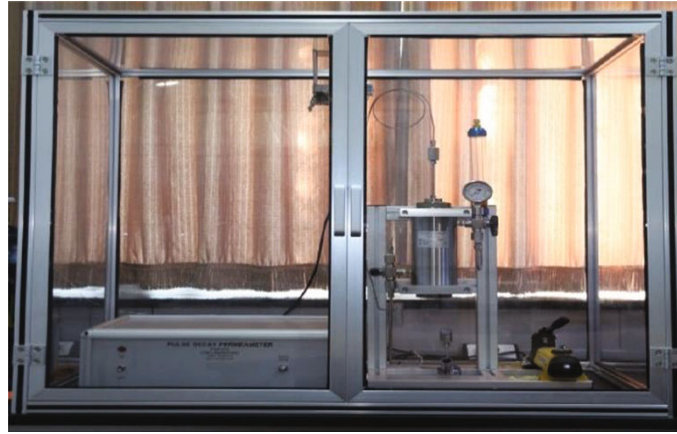
FIGURE 1: PDP200 permeability measurement apparatus (pressure decay method).
