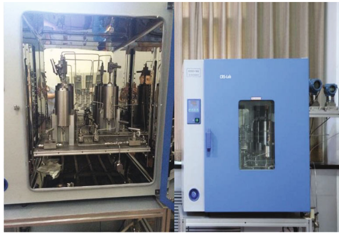
FIGURE 2: PTM permeability measurement apparatus (pressure transmission decay method).
