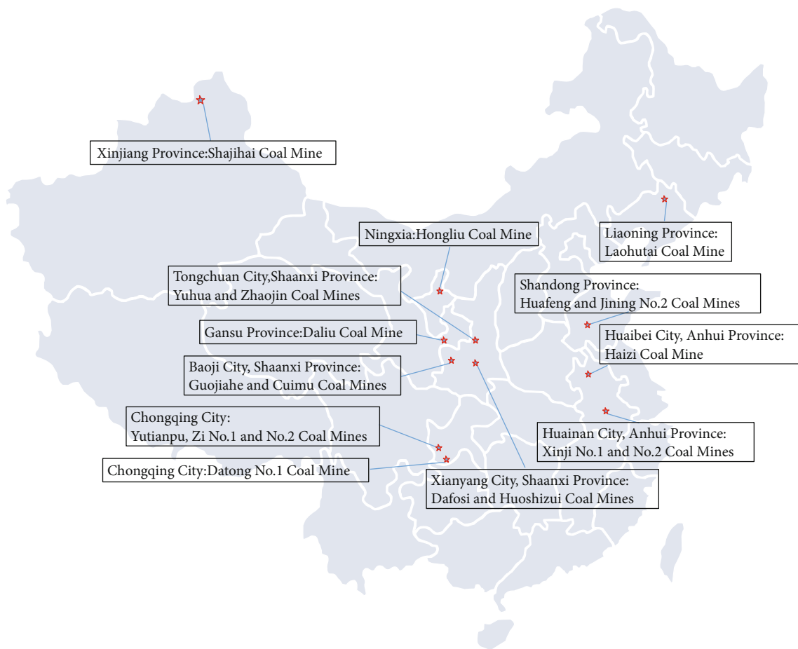
FIGURE 2: Distribution of bed separation water inrush accidents in China.
