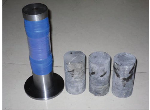
FIGURE 6: Postpeak rock specimen for measurement.
