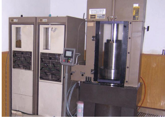
FIGURE 2: MTS815.02 electrohydraulic servocontrolled rock mechanics testing system.
