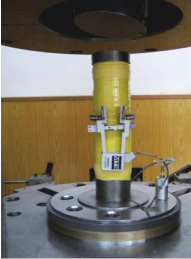
FIGURE 5: Rock specimen placed on MTS815 system.
