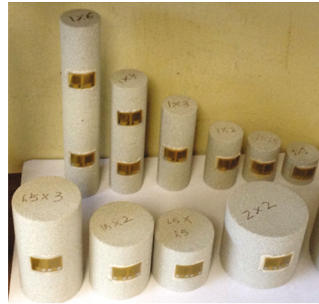
FIGURE 4: Core samples with the strain gauges attached.
