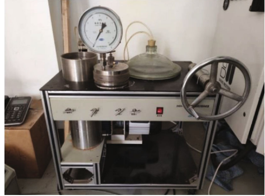
FIGURE 4: The vacuum saturation apparatus.
