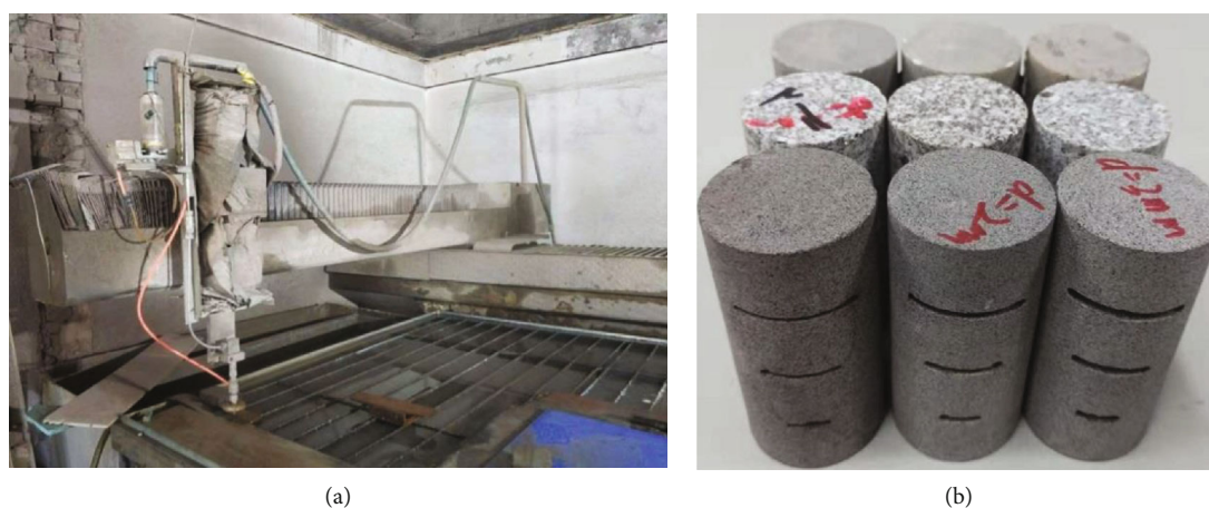
FIGURE 3: Preparation of rock sample with preexisting flaws: (a) the water-jet machine; (b) rock samples of different lithology with flaws used in the test.
