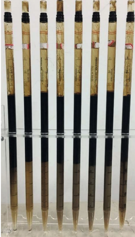
FIGURE 1: Phase behavior of surfactant and crude oil. The salinity from left to right is 0, 0.25%, 0.5%, 0.75%, 1%, 2%, 3%, and 5%.
