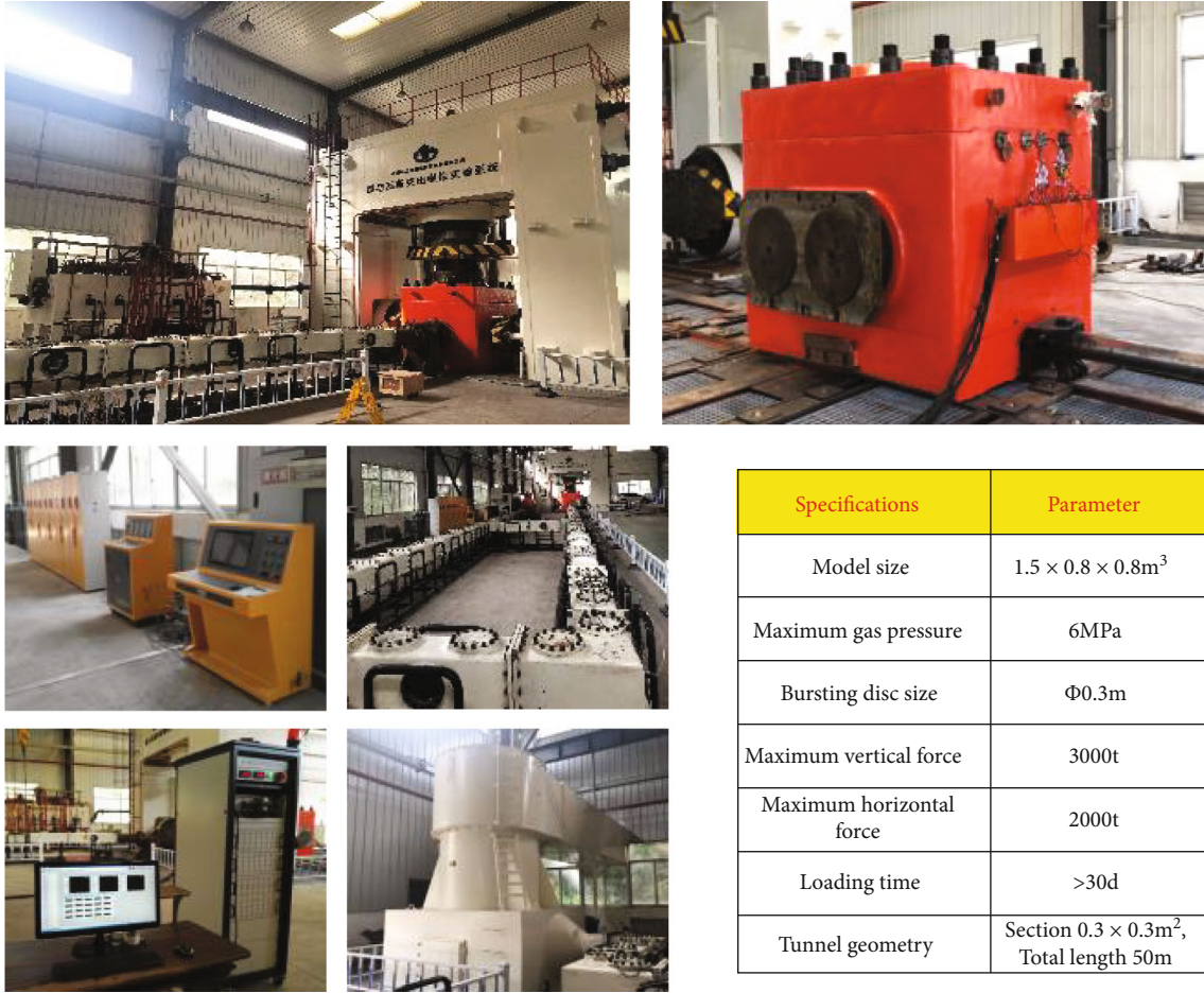
FIGURE 1: Coal and gas outburst simulation experiment system.
