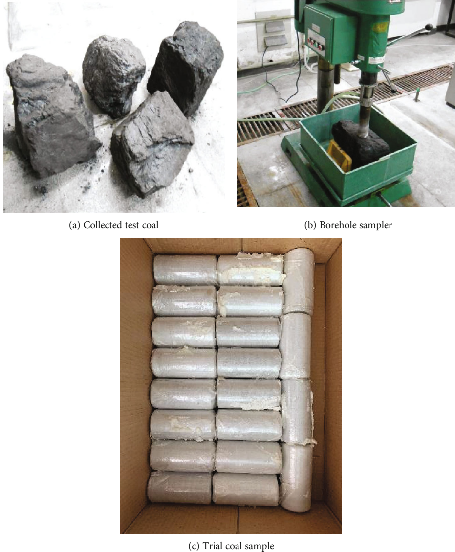
FIGURE 3: The collected coal, borehole sampler, and trial coal sample.
