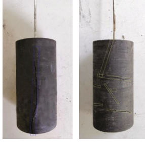
FIGURE 9: Crack propagation paths for the coal samples fractured by (1) water and (2) ScCO 2 .
