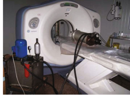
FIGURE 1: Portable dynamic loading equipment and CT scanner (reproduced from Fang et al. [24]).
