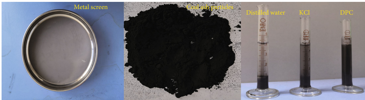
FIGURE 6: Test on coal ash particle expansion with different fluids.
