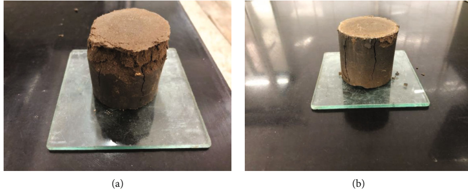
FIGURE 4: Destruction image of unconfined compression specimen: (a) plain soil; (b) cement-modified soil (mixed with 3%).
