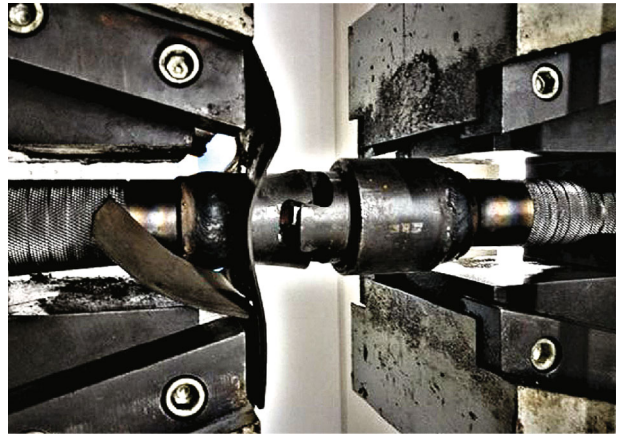
FIGURE 8: Tensile performance test of the bionic drill pipe.
