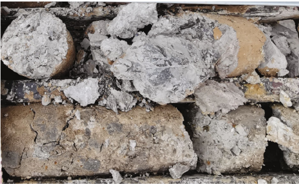
FIGURE 2: Rock core of the upper “soft” completely weathered siliceous rock.
