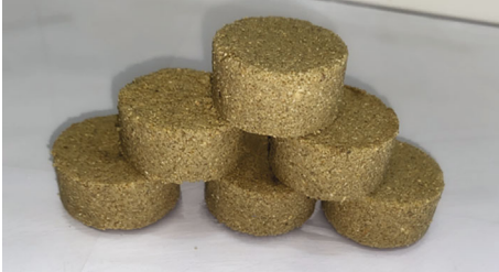
FIGURE 1: The prepared ice-rich frozen sandy soil specimen.
