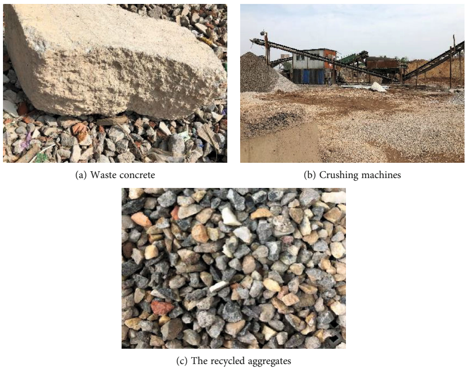
FIGURE 2: The recycled concrete aggregates used in the tests.
