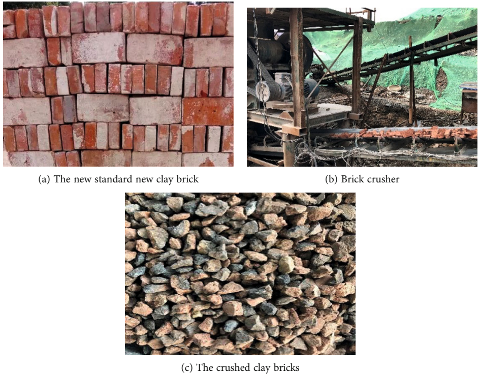
FIGURE 1: The crushed clay brick aggregates used in the tests.
