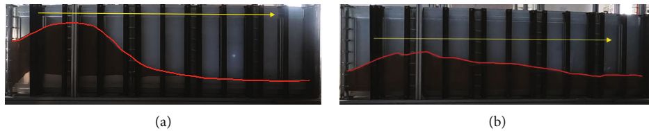
FIGURE 10: Configuration of 20/40 mesh quartz sand with different fracturing fluid viscosities: (a) viscosity of 3 mPa s and (b) viscosity of 5 mPa s.
