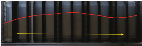
FIGURE 15: 20/40 mesh ceramsite sand embankment configuration with sand-carrying liquid viscosity of 15 mPa s.
