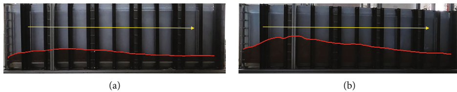
FIGURE 5: Layout diagram of sand dune with different sand ratios: (a) sand ratio of 6% and (b) sand ratio of 8%.
