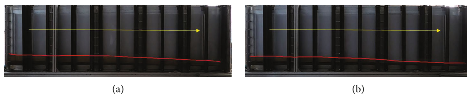
FIGURE 13: Sand embankment placement morphology in the evaluation experiment of tight gas layer: (a) the 12th group experiment and (b) the 13th group experiment.
