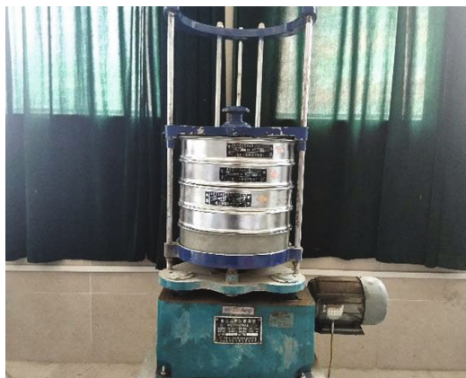
FIGURE 1: Screening marine soft soil.
