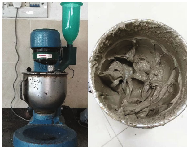
FIGURE 2: Mixing the components.
