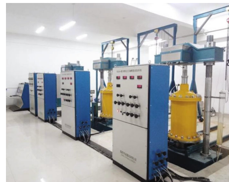
FIGURE 2: Triaxial testing system (SZLB-4).
