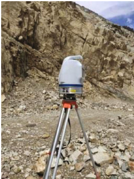
FIGURE 2: Placement of 3D laser scanner.
