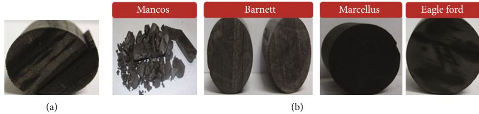
FIGURE 4: (a) Barnett shale sample after one week of spontaneous imbibition in distilled water [71]. (b) Imbibition testing results from Morsy and Sheng [66].
