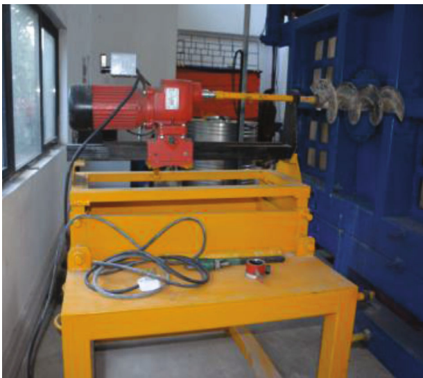
FIGURE 5: The tunnel excavation simulation system [42].
