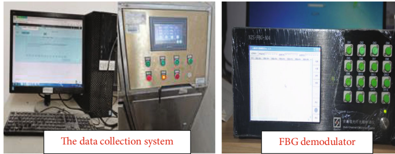
FIGURE 7: The intelligent data collection system [43].
