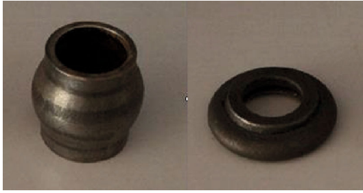
FIGURE 13: The yielding pipe before and after work.
