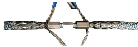
FIGURE 16: Use diagram of ultra-high-pressure hose and antistripping chain.
