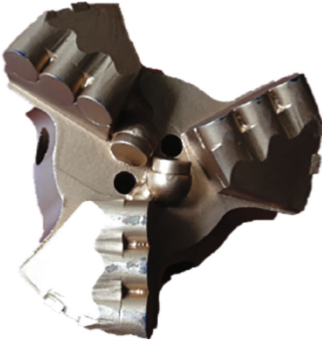
FIGURE 8: Schematic diagram of diamond compact drill bit.
