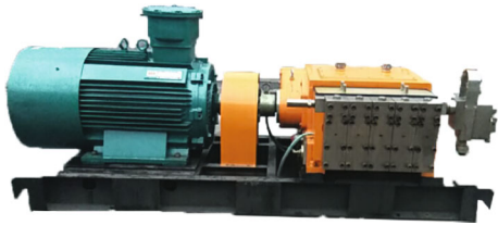
FIGURE 13: Schematic diagram of ultra-high-pressure clean water pump.
