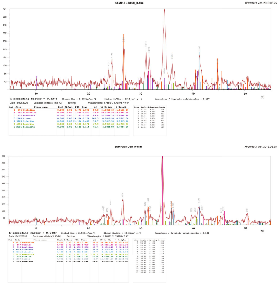
FIGURE 8: XRD results for samples BASH and OBA.
