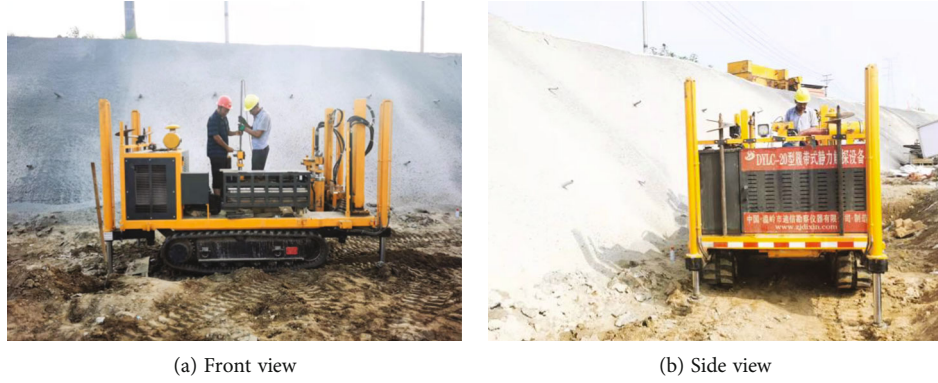
FIGURE 4: Work diagram of field static penetration test.
