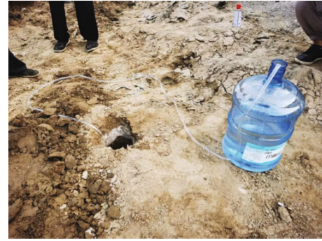
FIGURE 3: Field water injection operation chart.
