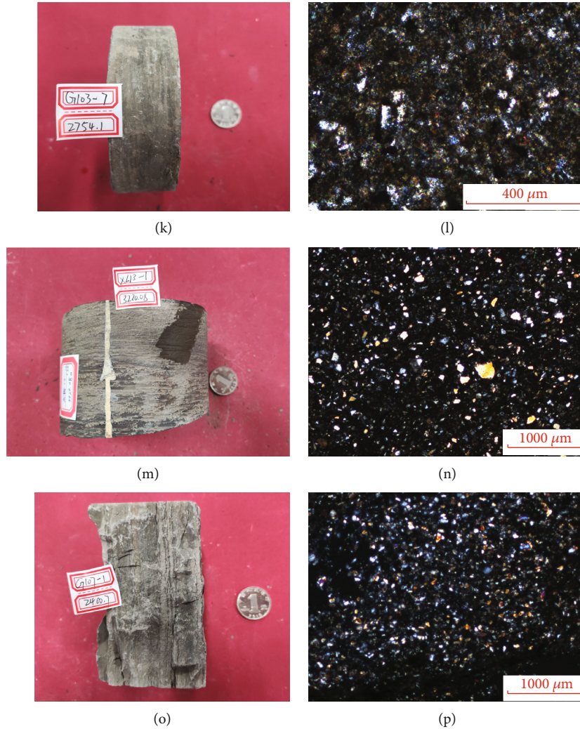
FIGURE 8: (a, b) Calcareous-rich MS, well XL25x, 3540.65 m; (c, d) calcareous-rich MS, well G24, 2617.00 m; (e, f) calcareous MS, well XL25x, 3538.41 m; (g, h) clay MS, well B11x, 3543.90 m; (i, j) clay MS, well G34, 2517.56 m; (k, l) clay-rich MS, well G103, 2754.10 m; (m, n) felsic MS, well XL13, 3220.08 m; (o, p) felsic-rich MS, well G107, 2400.70 m.
